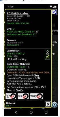
If you want to track specific OGN Device IDs, your 'Buddies', enter each Device ID in the box called 'Show specific OGN Device IDs'. Separate each Device ID with a '/'.For example XCG640000/XCG640001. You can also use a wildcard. For example to see all XCGuide users, at any distance, simply enter XCG\*.
