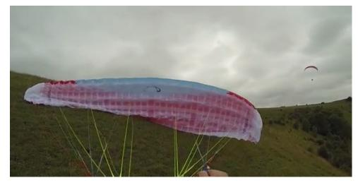
A useful technique that work well is to set up square to the wind, but take one large step up the slope – the effect on the 'wall' will be to raise the downslope side and counter any
